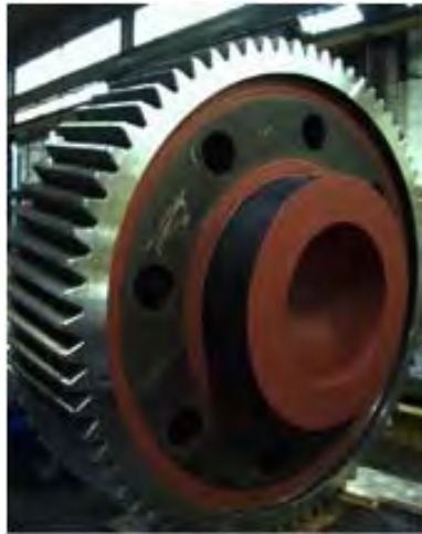
Figure 12. Example of a larger gear designed as a welded construction
