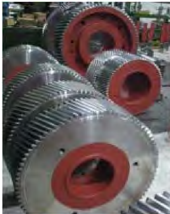
Figure 10. Smaller gears made as a solid structure, no weldments necessary
