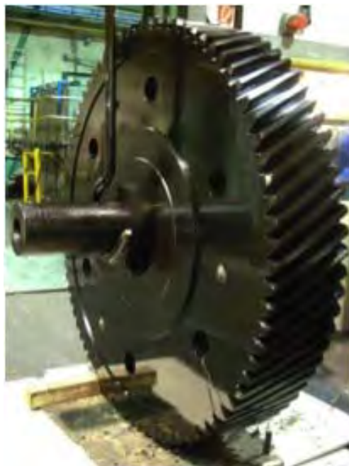
Figure 22. Example of different possible charging method (vertical charging)
