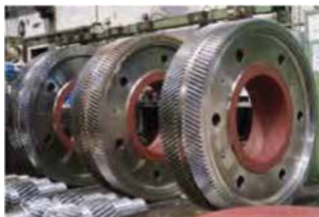
Figure 9: Medium gears that have been made as a solid structure
