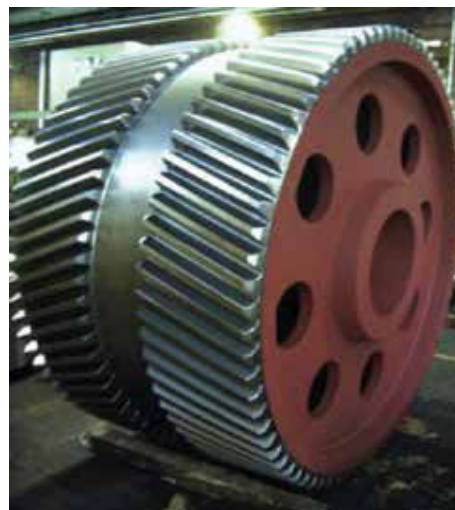
Figure 11: Example of a larger gear designed as a welded construction
